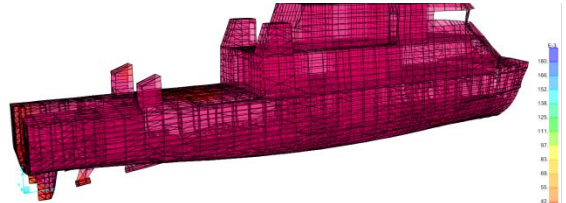
Figure 17 – Deformation (mm) at 29.73 Hz condition
