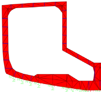
Figure 3 - Aft frame – Hull bottom restraints
